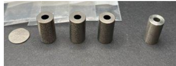
Zirconium Hydride 1.59 samples next to Zircaloy-4 control
