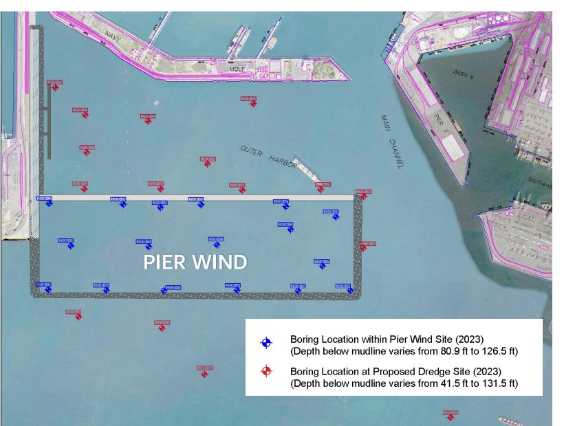
Performed 36 borings to get soil parameters. Information is used to inform:
