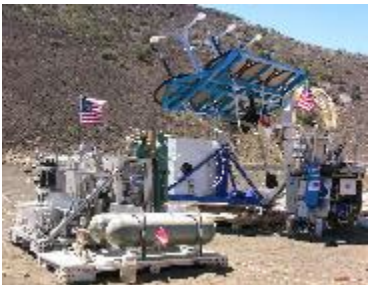
Oxygen from Mare Regolith – Carbothermal Reduction (2010)
