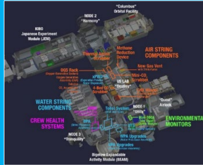
Upgraded ISS Urine Processor Distillation Assembly (85% water recovery)
