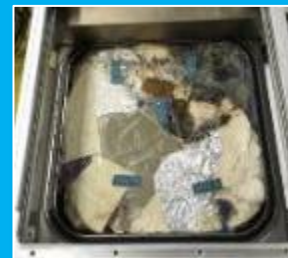
Trash Processing and Compaction System (compacted tile in ground prototype)
