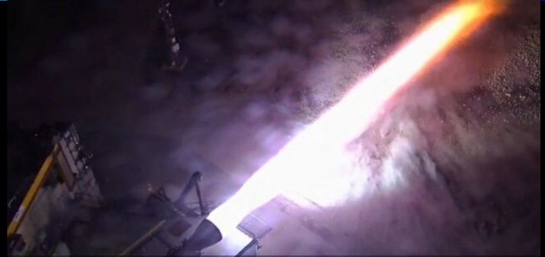
The 281-second throttle test demonstrated the engine's ability to meet the demands of a descent burn to the lunar surface. Credit: SpaceX
