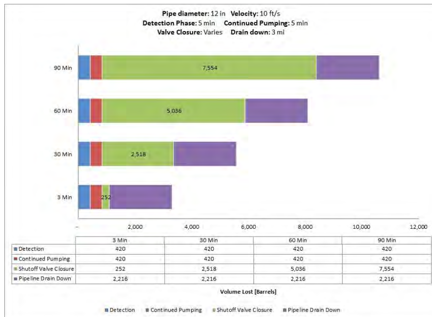
Fig. A-60. 12 Inch Pipe Diameter, 10 ft/s, 1480 psi MAOP, 1000 Feet Elevation Change.
