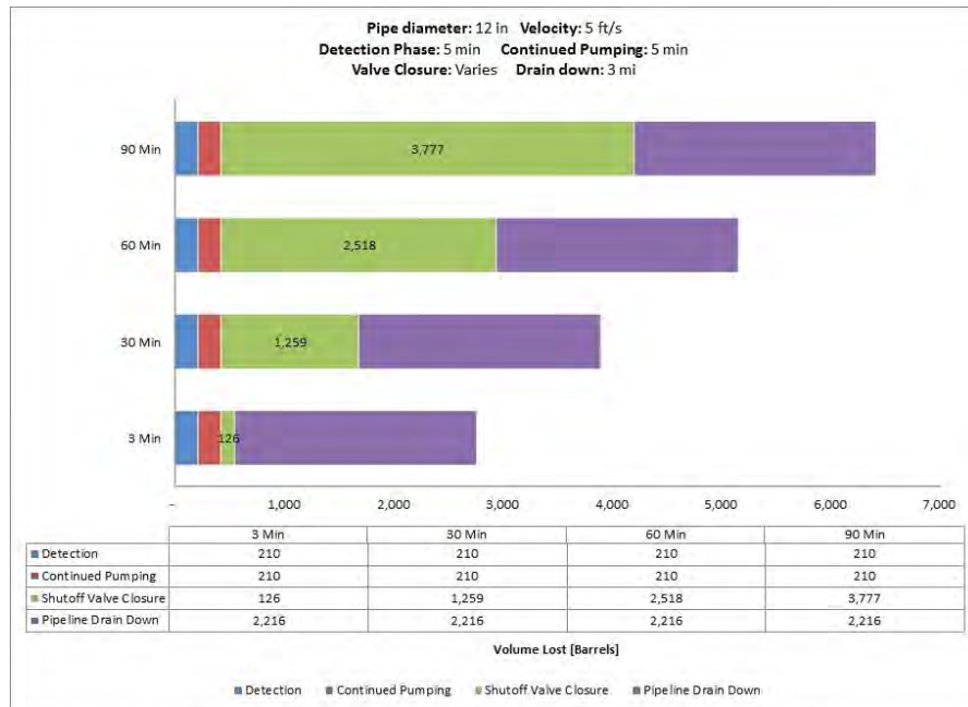
Fig. A-43. 12 Inch Pipe Diameter, 5 ft/s, 1200 psi MAOP, 100 Feet Elevation Change.
