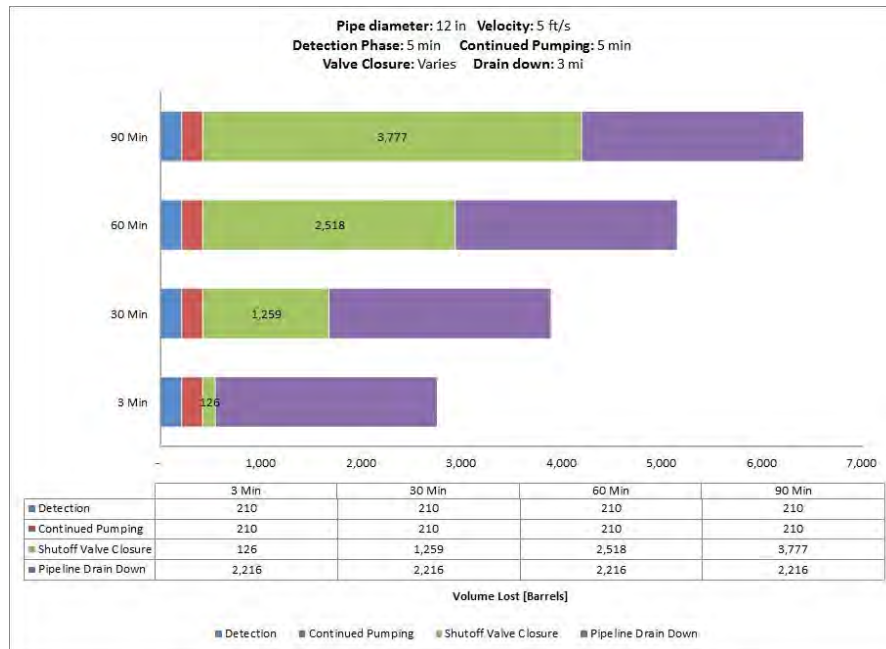
Fig. A-47. 12 Inch Pipe Diameter, 5 ft/s, 1480 psi MAOP, 500 Feet Elevation Change.
