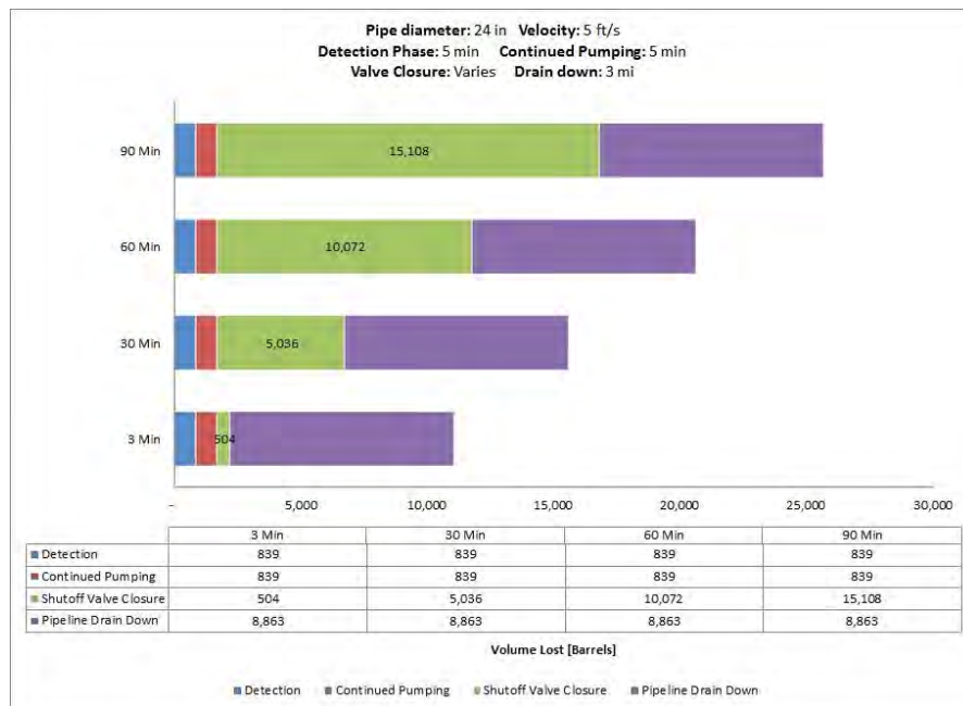
Fig. A-116. 24 Inch Pipe Diameter, 5 ft/s, 1200 psi MAOP, 500 Feet Elevation Change.
