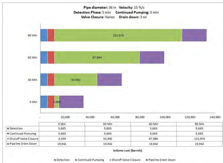
Fig. 3.84. Case Study 8C – Discharge volumes for a 36-in. hazardous liquid pipeline with a 400 psig MAOP and an elevation change of 1,000 ft with a 3, 30, 60, and 90 minutes block valve closure phase.
