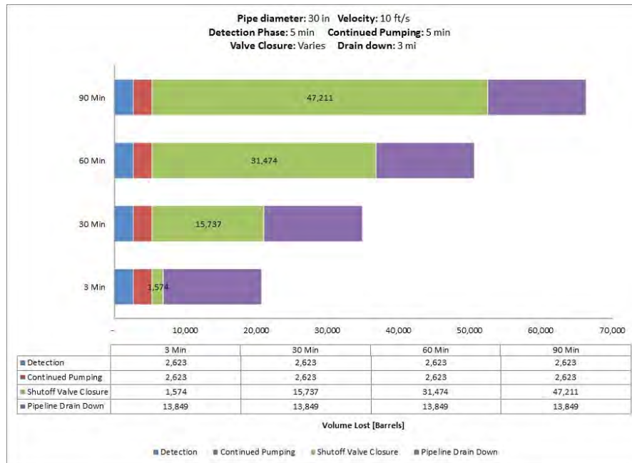
Fig. A-157. 30 Inch Pipe Diameter, 10 ft/s, 400 psi MAOP, 100 Feet Elevation Change.
