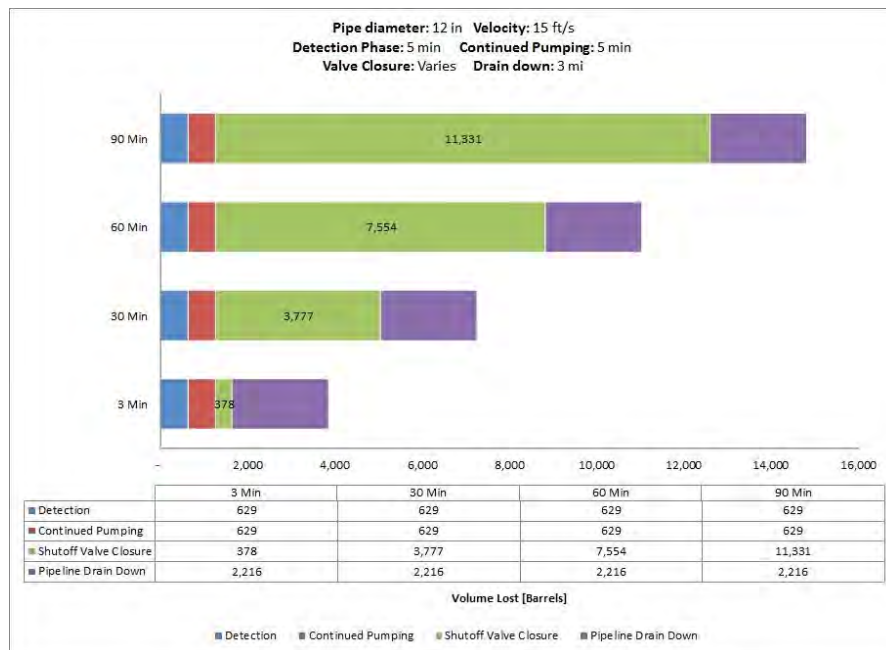
Fig. A-64. 12 Inch Pipe Diameter, 15 ft/s, 800 psi MAOP, 100 Feet Elevation Change.
