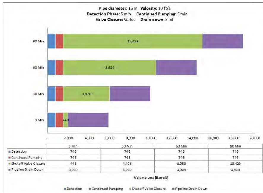
Fig. A-92. 16 Inch Pipe Diameter, 10 ft/s, 1200 psi MAOP, 500 Feet Elevation Change.
