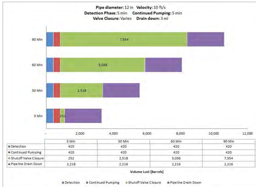
Fig. A-53. 12 Inch Pipe Diameter, 10 ft/s, 800 psi MAOP, 500 Feet Elevation Change.
