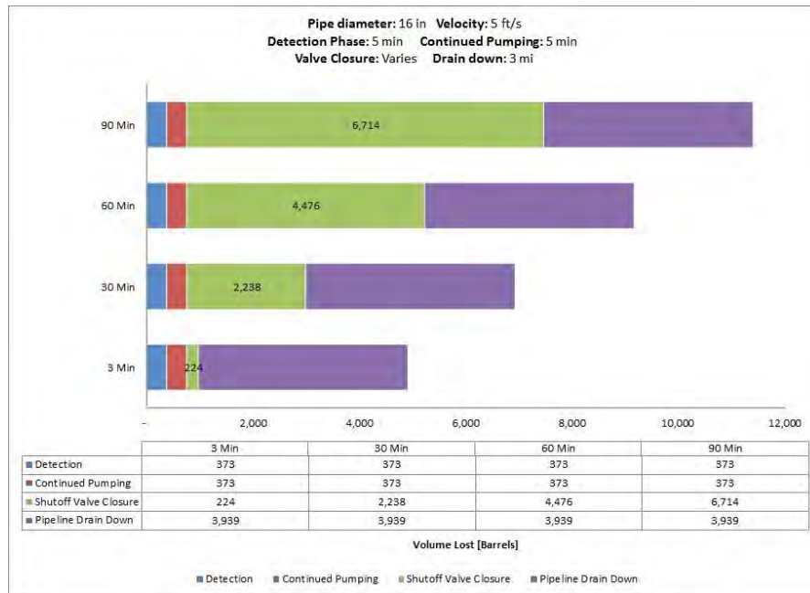
Fig. A-81. 16 Inch Pipe Diameter, 5 ft/s, 1200 psi MAOP, 1000 Feet Elevation Change.
