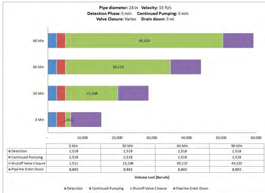
Fig. A-143. 24 Inch Pipe Diameter, 15 ft/s, 1480 psi MAOP, 500 Feet Elevation Change.
