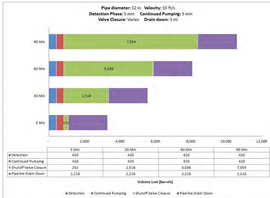
Fig. A-59. 12 Inch Pipe Diameter, 10 ft/s, 1480 psi MAOP, 500 Feet Elevation Change.
