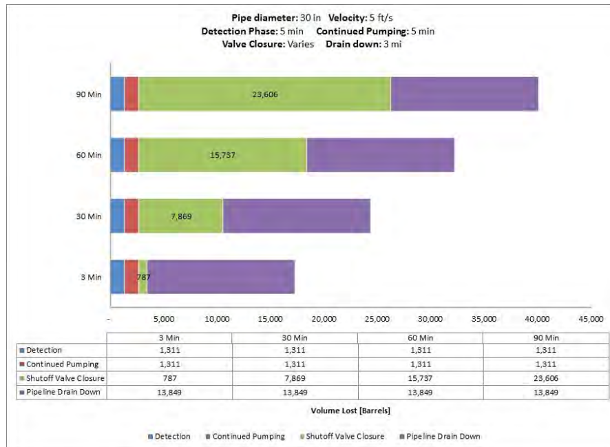
Fig. A-155. 30 Inch Pipe Diameter, 5 ft/s, 1480 psi MAOP, 500 Feet Elevation Change.
