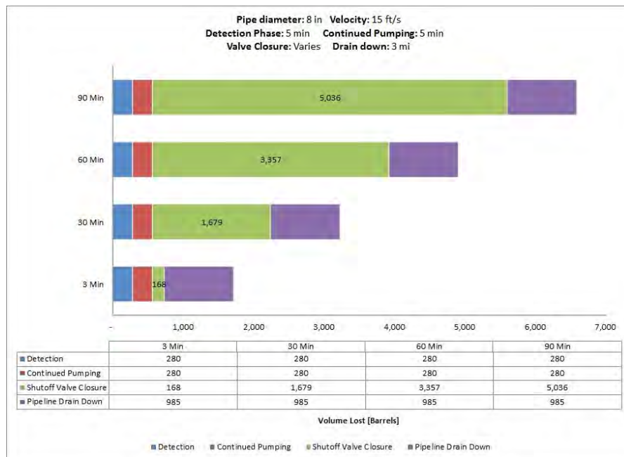
Fig. A-32. 8 Inch Pipe Diameter, 15 ft/s, 1200 psi MAOP, 500 Feet Elevation Change.
