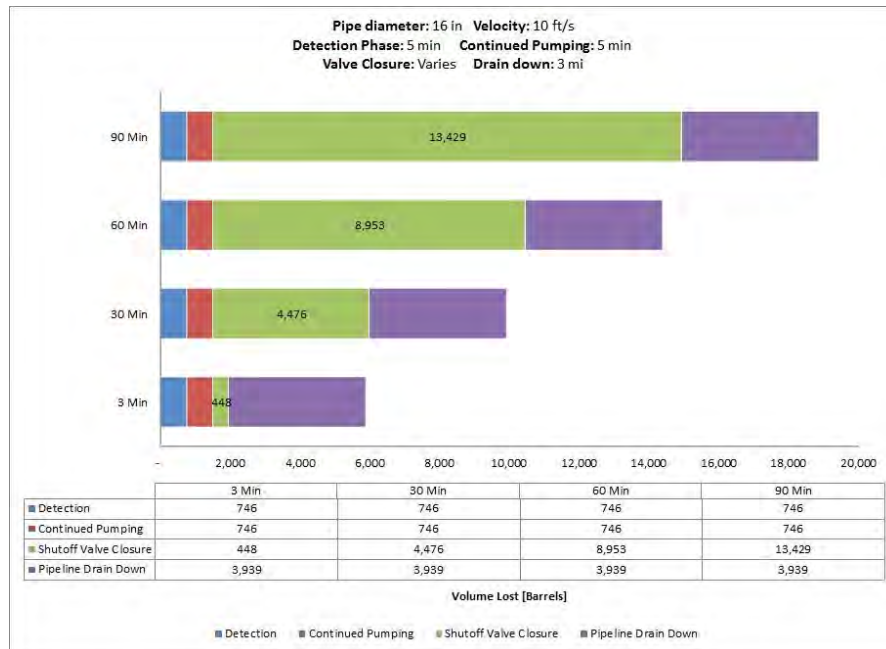
Fig. A-89. 16 Inch Pipe Diameter, 10 ft/s, 800 psi MAOP, 500 Feet Elevation Change.
