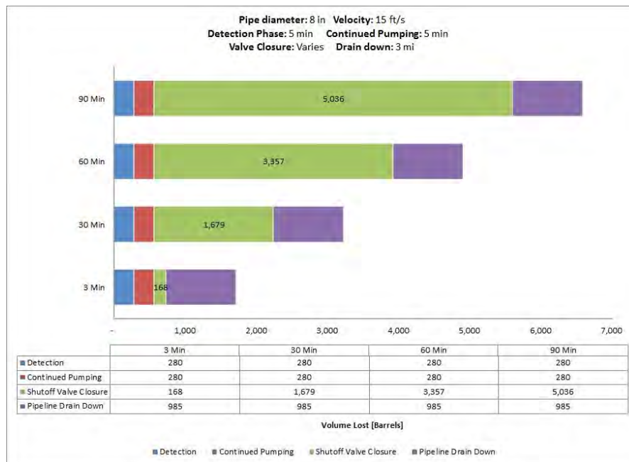
Fig. A-36. 8 Inch Pipe Diameter, 15 ft/s, 1480 psi MAOP, 1000 Feet Elevation Change.
