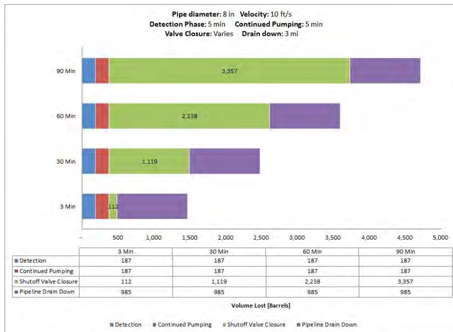
Fig. A-22. 8 Inch Pipe Diameter, 10 ft/s, 1480 psi MAOP, 100 Feet Elevation Change.
