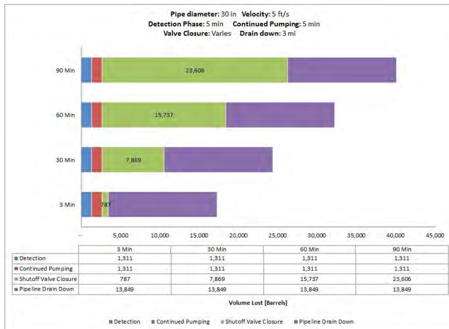
Fig. A-150. 30 Inch Pipe Diameter, 5 ft/s, 800 psi MAOP, 1000 Feet Elevation Change.
