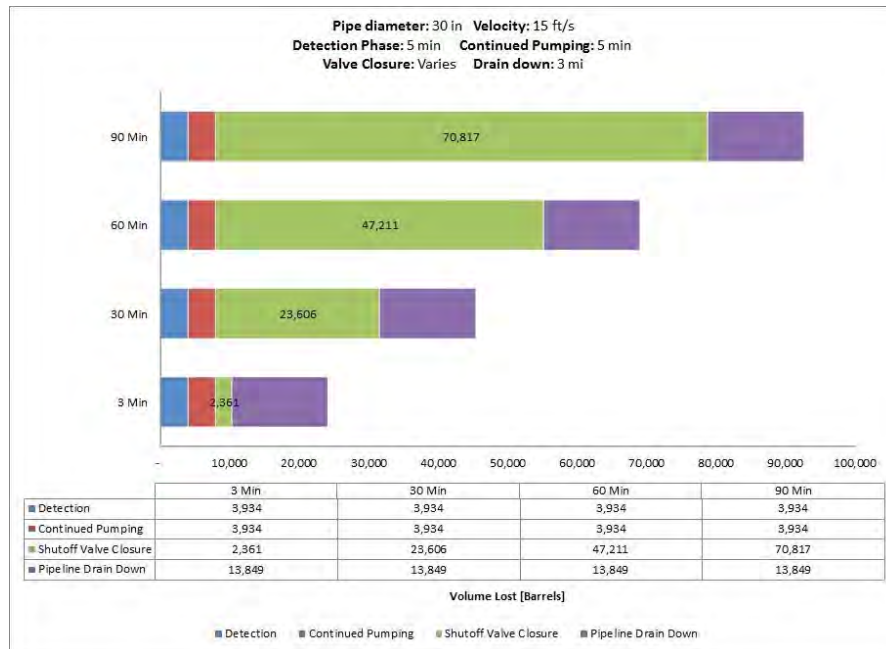
Fig. A-171. 30 Inch Pipe Diameter, 15 ft/s, 400 psi MAOP, 1000 Feet Elevation Change.
