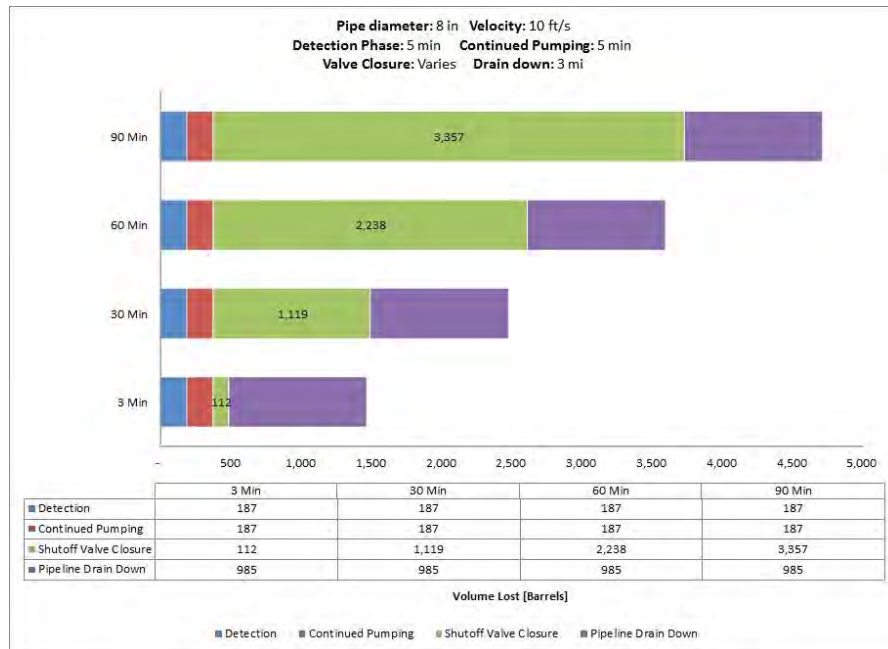
Fig. A-19. 8 Inch Pipe Diameter, 10 ft/s, 1200 psi MAOP, 100 Feet Elevation Change.
