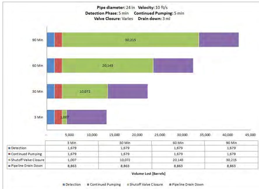
Fig. A-129. 24 Inch Pipe Diameter, 10 ft/s, 1200 psi MAOP, 1000 Feet Elevation Change.
