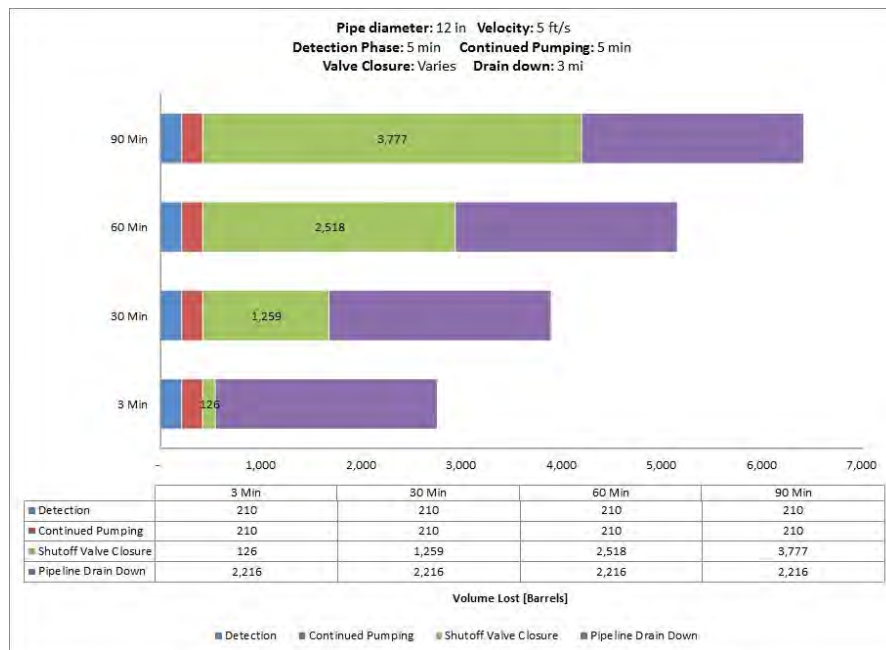
Fig. A-38. 12 Inch Pipe Diameter, 5 ft/s, 400 psi MAOP, 500 Feet Elevation Change.
