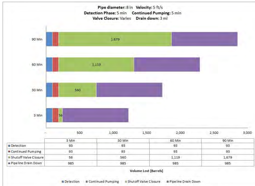
Fig. A-5. 8 Inch Pipe Diameter, 5 ft/s, 800 psi MAOP, 500 Feet Elevation Change.
