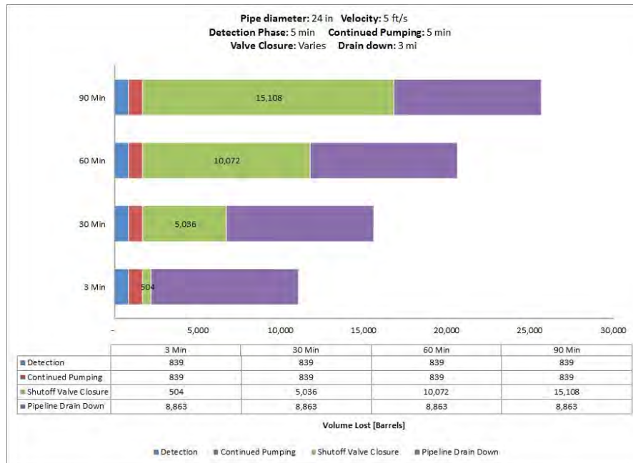
Fig. A-111. 24 Inch Pipe Diameter, 5 ft/s, 400 psi MAOP, 1000 Feet Elevation Change.
