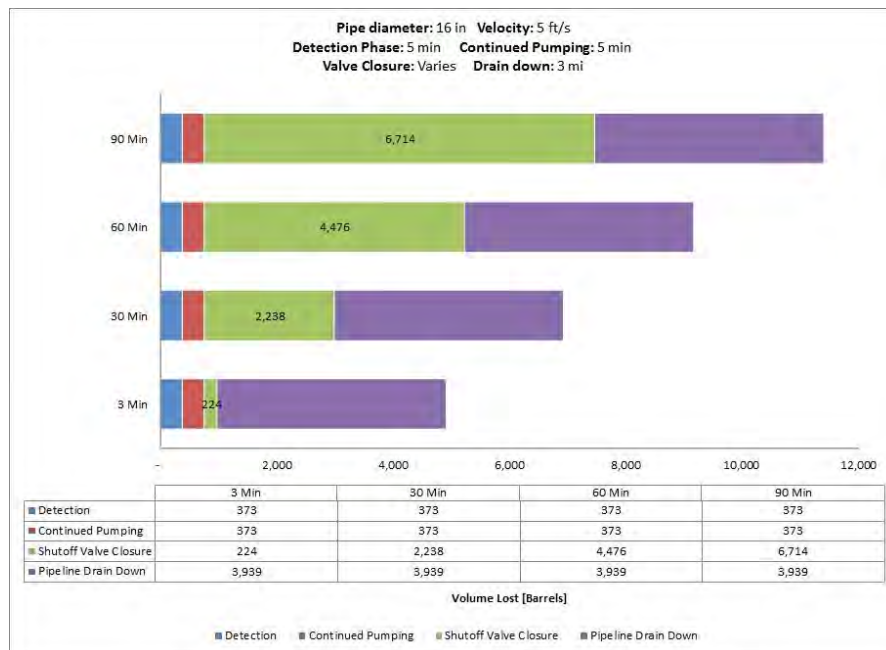
Fig. A-82. 16 Inch Pipe Diameter, 5 ft/s, 1480 psi MAOP, 100 Feet Elevation Change.
