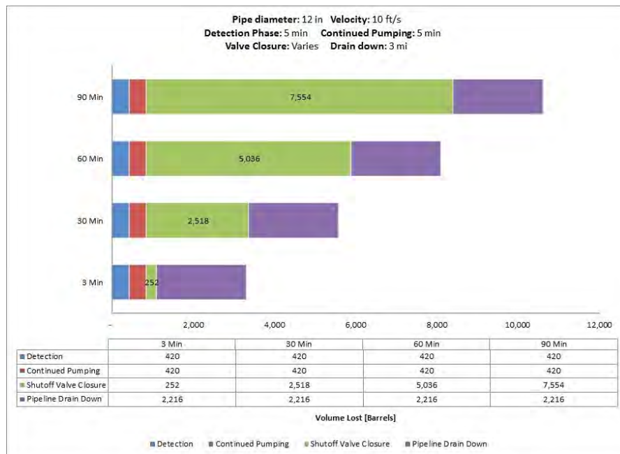
Fig. A-54. 12 Inch Pipe Diameter, 10 ft/s, 800 psi MAOP, 1000 Feet Elevation Change.
