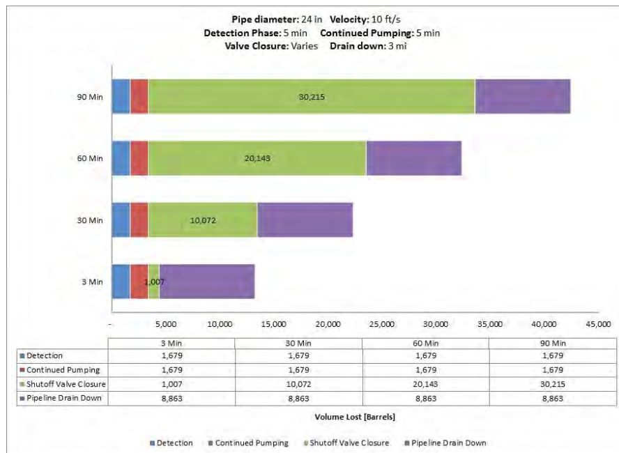
Fig. A-130. 24 Inch Pipe Diameter, 10 ft/s, 1480 psi MAOP, 100 Feet Elevation Change.
