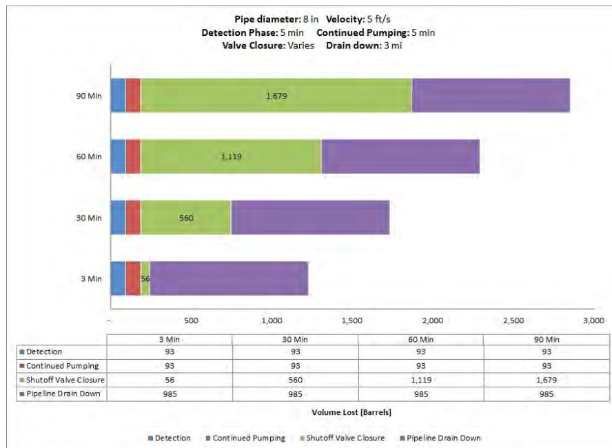
Fig. A-4.8 Inch Pipe Diameter, 5 ft/s, 800 psi MAOP, 100 Feet Elevation Change.
