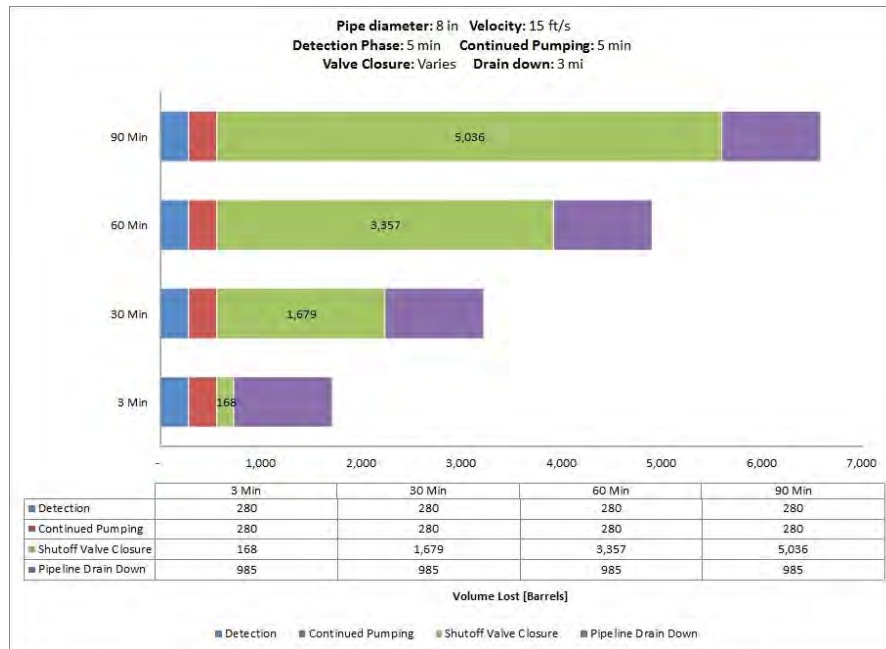
Fig. A-25. 8 Inch Pipe Diameter, 15 ft/s, 400 psi MAOP, 100 Feet Elevation Change.
