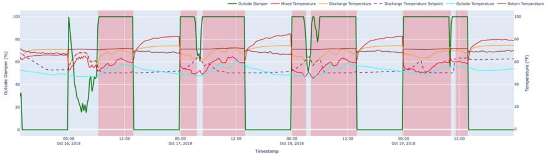
HVAC System Performance - Air Handling Unit 19 (Red highlights: Heating Valve Leaking)
