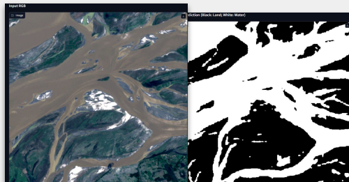
Model fine-tuned to segment the extent of floods on Sentinel-2
