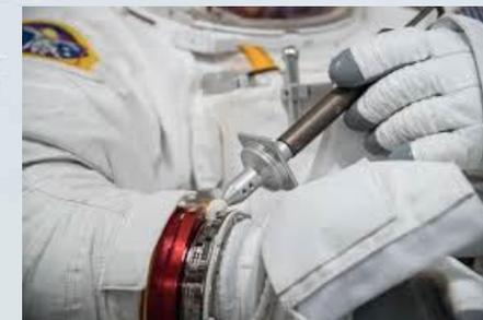
EVA Swab On Ground Testing of the EMU Wrist Joint Sampling. NASA
