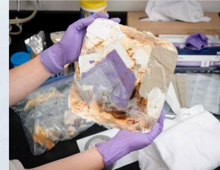
Sample trash tile, compressed to  $<1/8$ th of the original volume, by the Heat Melt Compactor. NASA Ames Research Center/Dominic Hart
